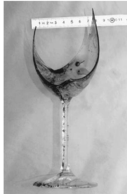
Fig. 4 The wineglass recovered from the table including an intact basis and stem but a broken goblet which forms two long and dagger-like fragments protruding upwards. The distance of 7.1 cm between the tips of the goblet corresponds exactly to the one between the beginnings of the skin notches, which were caused by the tips moving tangentially to the skin surface (compare Fig. 1)
